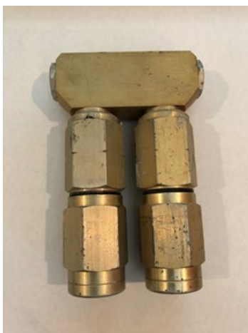
Figure 29. Trunk splice removed from network.
