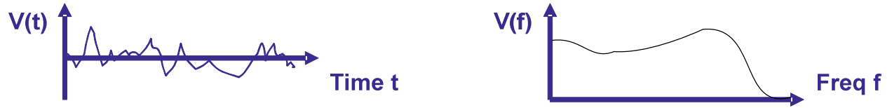
Fig. 3c- Semi-Additive White Gaussian Noise in Frequency Domain
