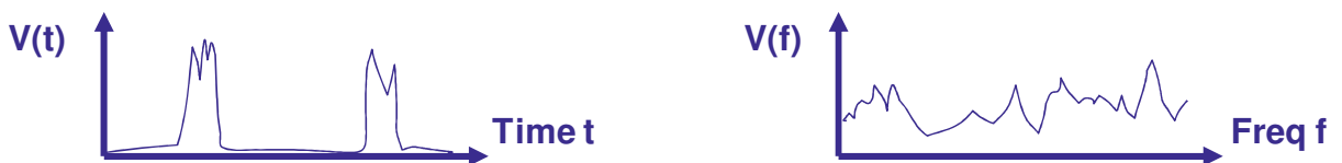
Fig. 5- Example of Impulse Noise in the Time Domain and Frequency Domain
